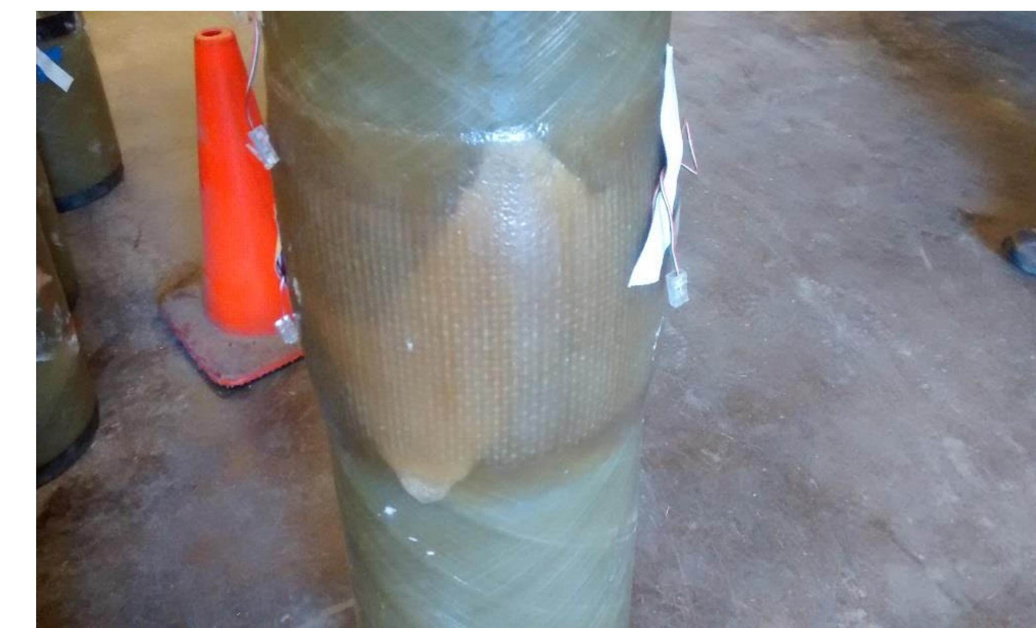
Figure 5. Delamination of the external wrap on the butt joint.
