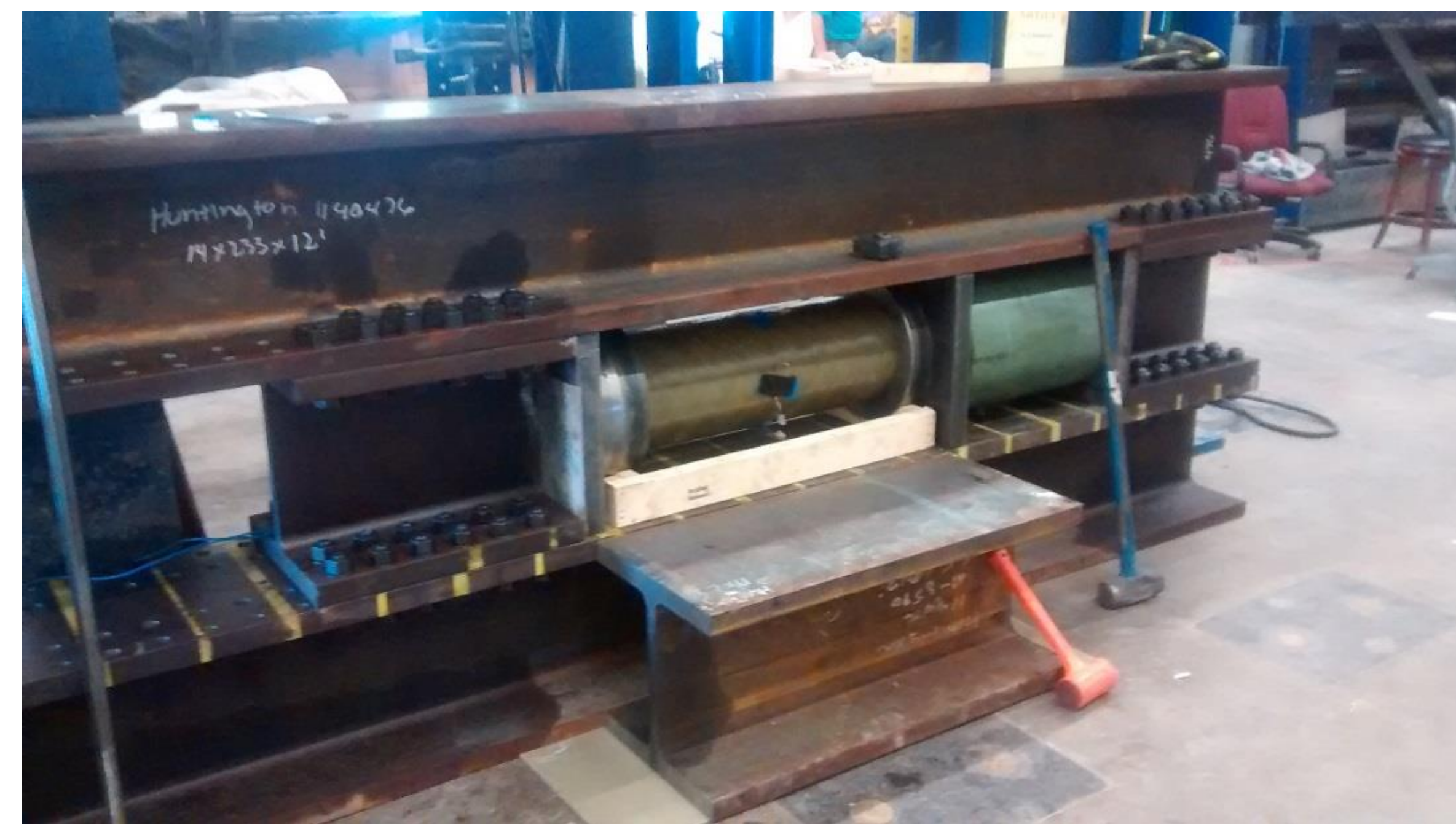
Figure 2. Burst pressure testing of fiber wound pipe.
